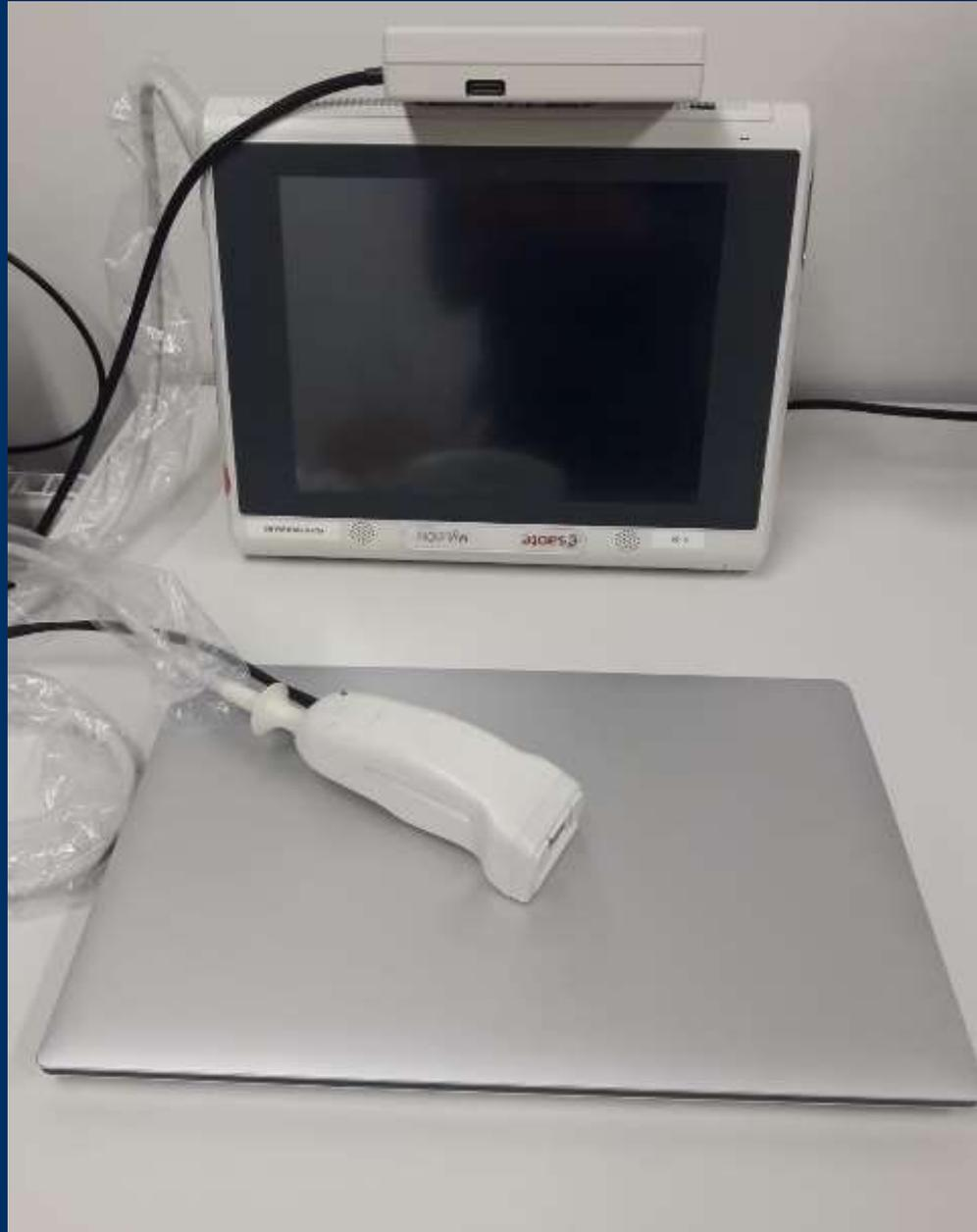
The portable photo acoustic-ultrasound imaging system and the hand-held probe.
